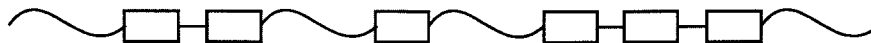
Figure 2 Schematic representation of TΦT-PTMO copolymers containing an extender: (□) TΦT unit; (—) extender; and (~~~~) PTMO.
